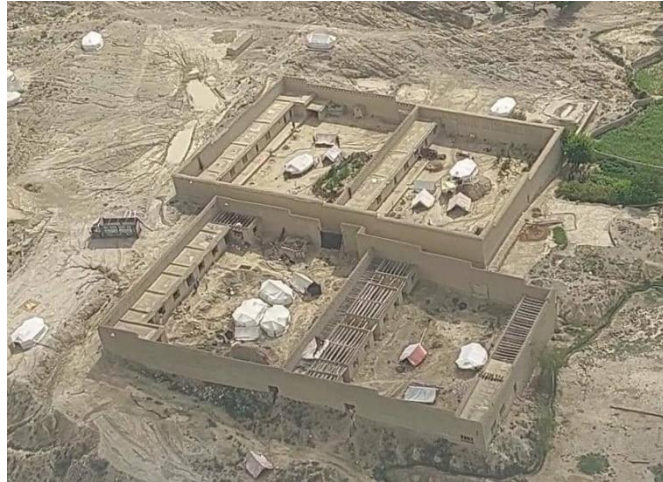
Figure 3-2. Four compounds as seen from the air. Note the construction of rooms along the perimeter wall with open spaces in the middle. Photo courtesy of Jago Boase, IOM.
